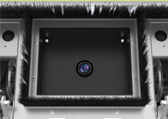
Shading brush bristles severely deformed
