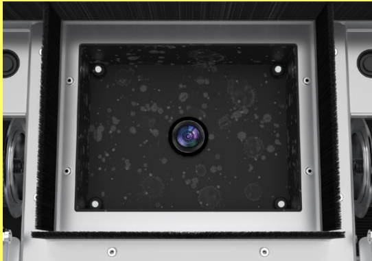
The inside of the exposure box and camera lens are stained
