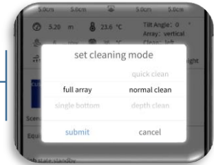
Custom cleaning mode Array/Single bottom Quick/Normal/Deep/Severe
